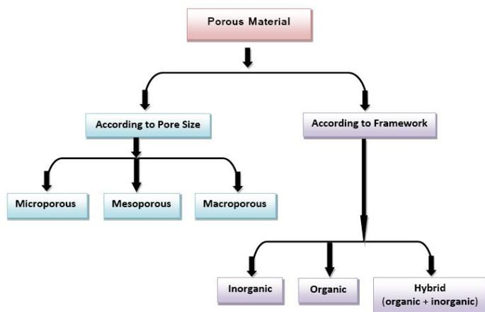
**Figure 3:** Classification of porous material according to pore size and build-up framework
