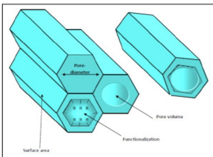
**Figure 5:** Pore geometry of mesoporous material
