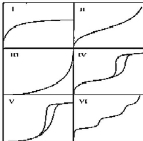
Figure 2: Types of adsorption isotherm according to IUPAC
