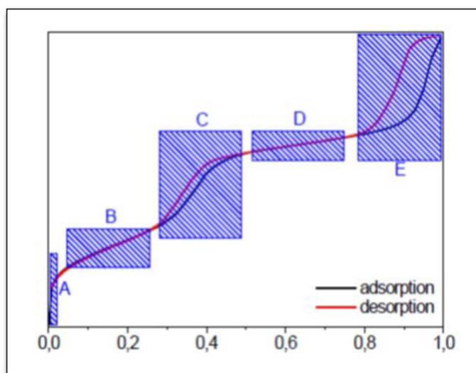
**Figure 4:** Typical isotherm for a bulk sample of mesoporous material
