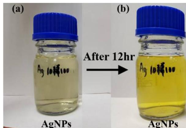
**Figure 4:** (a) Initial reaction solution with 1 mM silver nitrate. (b) Diluted reaction solution after 12 hours.
