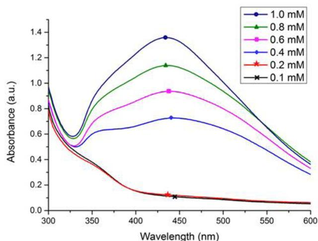
**Figure 2:** Absorbance spectra for reaction solutions produced using 1 ml of tea extract and silver nitrate concentrations of 0.1~1.0 mM.
