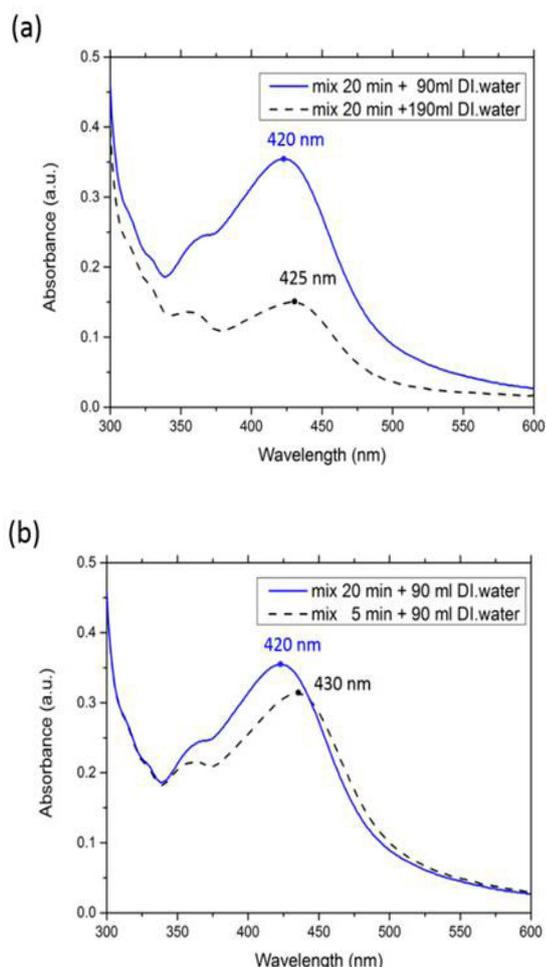
**Figure 6:** (a) Absorbance spectra of AgNP solutions diluted with 90 ml and 190 ml of DI water, respectively. (b) Absorbance spectra of diluted AgNP solutions with initial reaction times of 5 minutes and 20 minutes, respectively.
