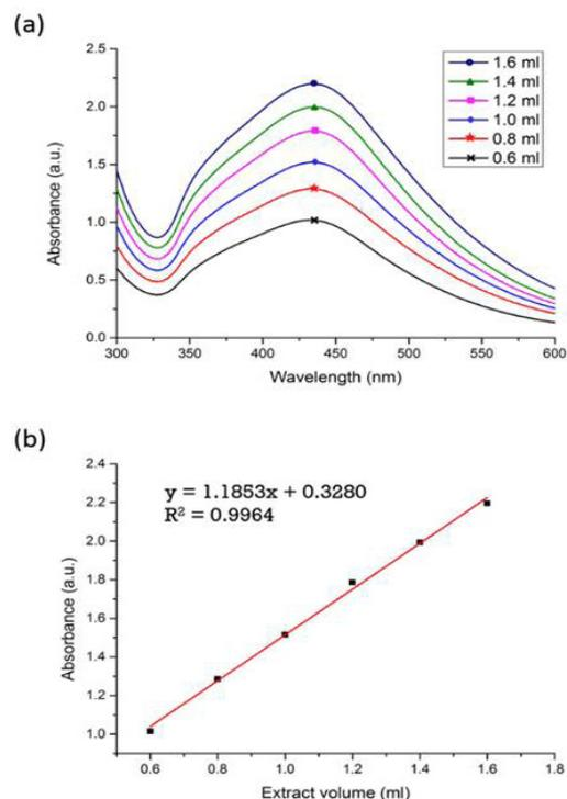
**Figure 3:** (a) Absorbance spectra for reaction solutions produced using silver nitrate concentration of 1 mM and tea extract volumes of 0.6 ~ 1.6 ml. (b) Regression analysis results for relationship between absorbance peak intensity and tea extract volume.
