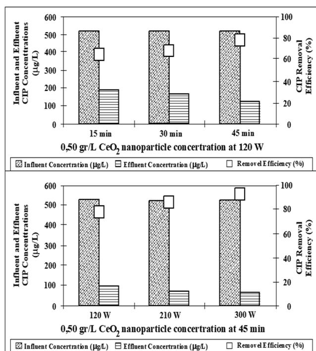
**Figure 4:** (a) CIP yields at different irradiation times at 120 W for 0.50 gr/L nano CeO<sub>2</sub> concentration at 25 °C and at a pH of 7.00. (b) CIP yields at different UV powers at 45 min for 0.50 gr/L nano CeO<sub>2</sub> concentration at 25 °C and at a pH of 7.00
