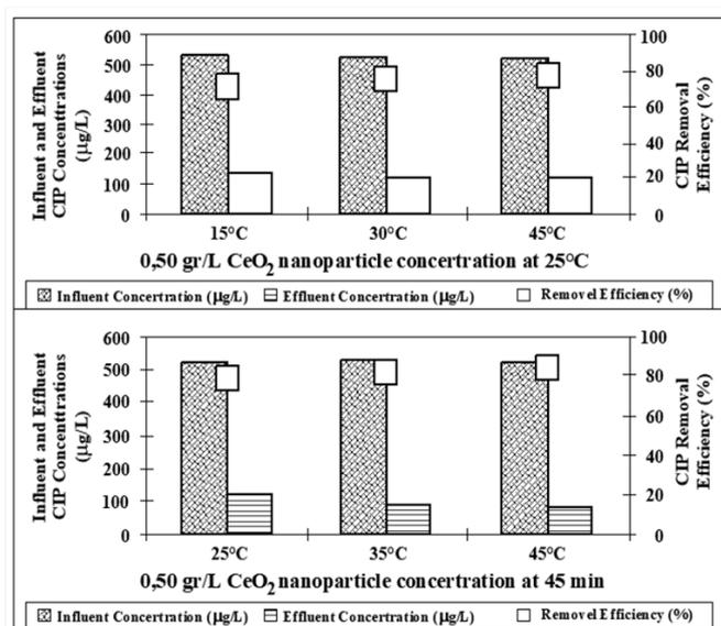
**Figure 3:** (a) CIP yields at different sonication times at 25 °C for 0.50 gr/L nano CeO<sub>2</sub> concentration at pH=7.00 at a frequency of 35 kHz and a power of 510 W. (b) CIP yields at different sonication temperatures at 45 min for 0.50 gr/L nano CeO<sub>2</sub> concentration at pH=7.00 at a frequency of 35 kHz and a power of 510 W
