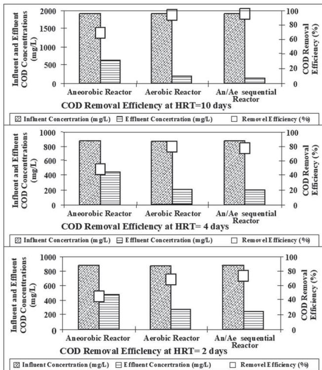
**Figure 1:** (a) COD concentrations and yields during the 10 days of HRT operation at 0.19 gr COD/L.day OLR. (b) COD concentrations and yields during the 4 days of HRT operation at 0.22 gr COD/L.day OLR. (c) COD concentrations and yields during the 2 days of HRT operation at 0.44 gr COD/L.day OLR.
