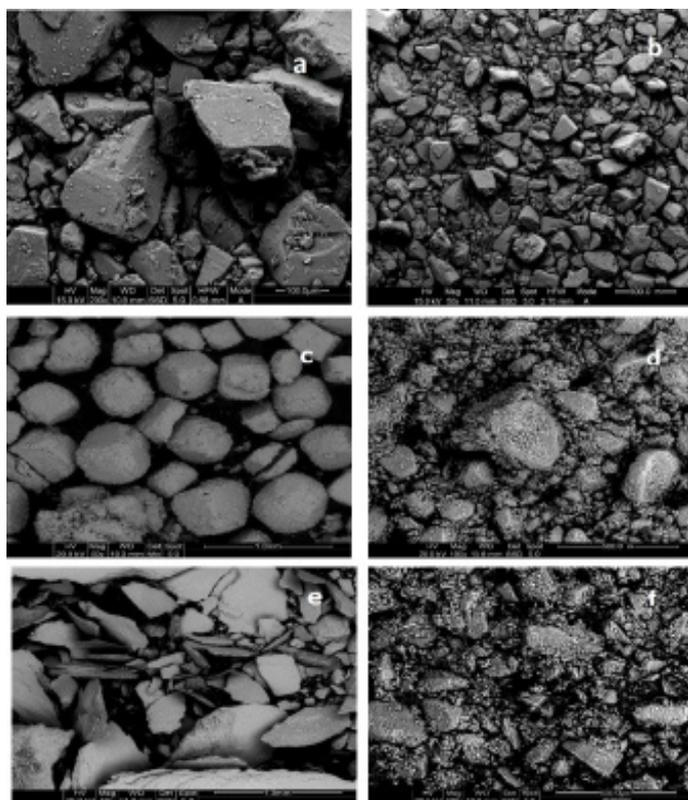
**Figure 1:** SEM images of (a)  $\alpha$ -Lactose monohydrate source material, (b) 6X trituration step of  $\alpha$ -Lactose monohydrate in  $\alpha$ -lactose monohydrate, (c) Sodium chloride source material, (d) 6X trituration step of Sodium chloride in  $\alpha$ -lactose monohydrate, (e) Calcium carbonate source material, (f) 6X trituration step of Calcium carbonate in  $\alpha$ -lactose monohydrate
