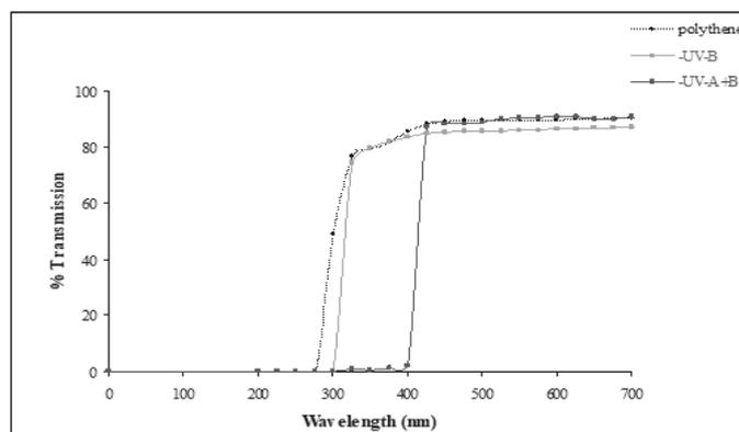
Figure 2: Transmission spectra of the UV-B and UV-B+A cutoff filters used on wire mesh cages for growing soybean plants under field conditions. The spectra between 200-700 nm by using an UV-visible spectrophotometer.
